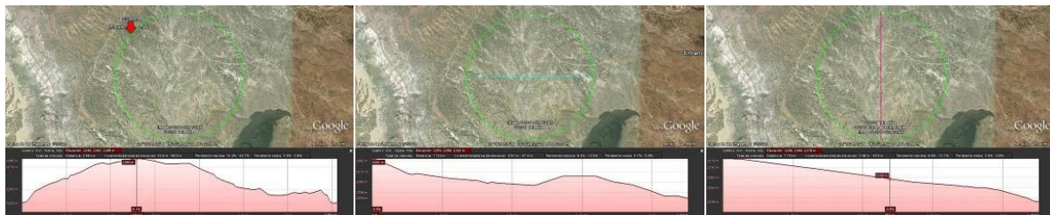
Figure 5.3: Left: altitude along the circle inside which CTA-North would be built. The maximum elevation is found at 2285 m (NW of the circle) and the minimum one at 2235 m, showing a maximum difference of 50 meters. Centre: altitude along the E-W diameter (in blue). The minimum elevation is 2251 m and the maximum one is 2280 m, showing a maximum difference of 30 meters. Right: altitude along the N-S diameter (in pink). The maximum elevation is 2279 m and the minimum one is 2236 m, showing a maximum difference of 45 meters 59 .
