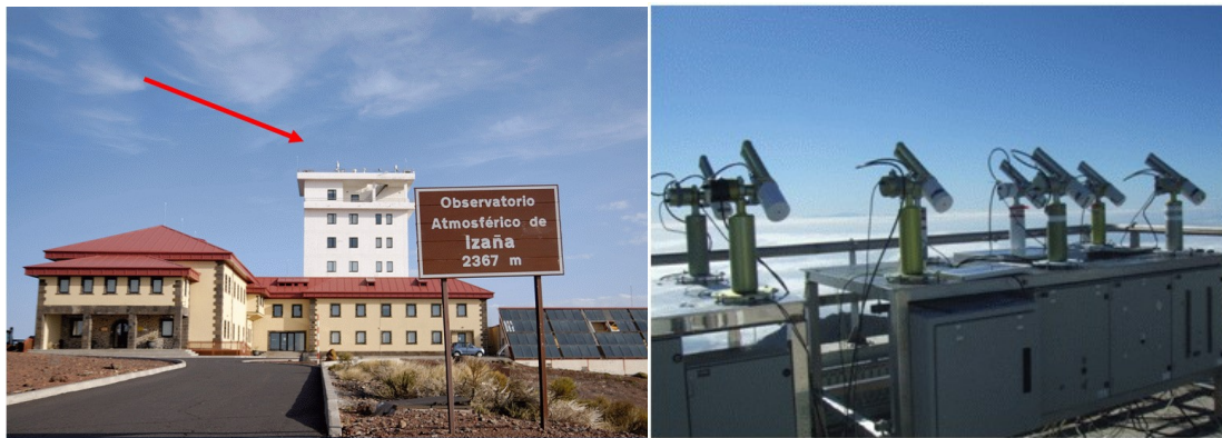
Figure 6.18 The Cimel sun photometer is a multichannel, automatic sun-and-sky scanning radiometer that measures the direct solar irradiance and sky radiance at the Earth's surface. Spectral range: 340, 380, 440, 500, 675, 870, 936, 1020, (and 1640) nm. At IZO, there are about 6 Cimel master working simultaneously.
